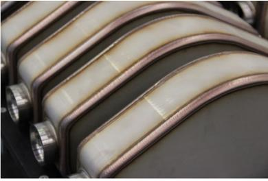
Critical temper colors: to prevent corrosion at a later stage, the reddish discoloration caused by welding must be removed by grit blasting.
