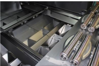
Injector blasting system: several Endress+Hauser flowmeters are ready to be cleaned in the blasting chamber.
