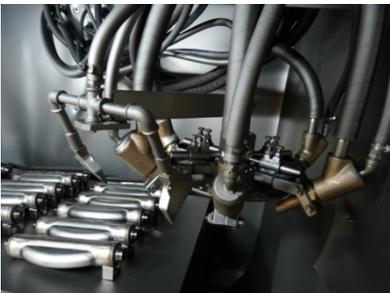
High pressure: the flowmeters are cleaned with six blasting nozzles, which blast the instruments at extreme velocity with ultra-fine stainless steel shot.
